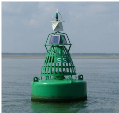
Figure 9 Example of numbering on floating AtoN
