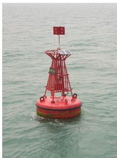
Figure 10 Example of Solar Panels installed on lateral mark
